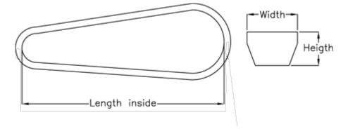
$\begin{array}{ll} \text{Datum Llength} = 6340 \\ \text{Height} & = 10 \\ \text{Length inside} & = 6300 \\ \text{Width} & = 17 \end{array}$
